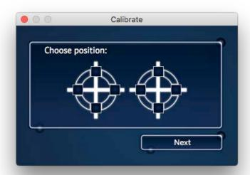
In the example shown here, the rudder / tail has moved to the right. After clicking on "Next", the StickMover will take the next position, which will also be specified accordingly. This process must be repeated 4 times (until all 4 servomotors have passed through).
